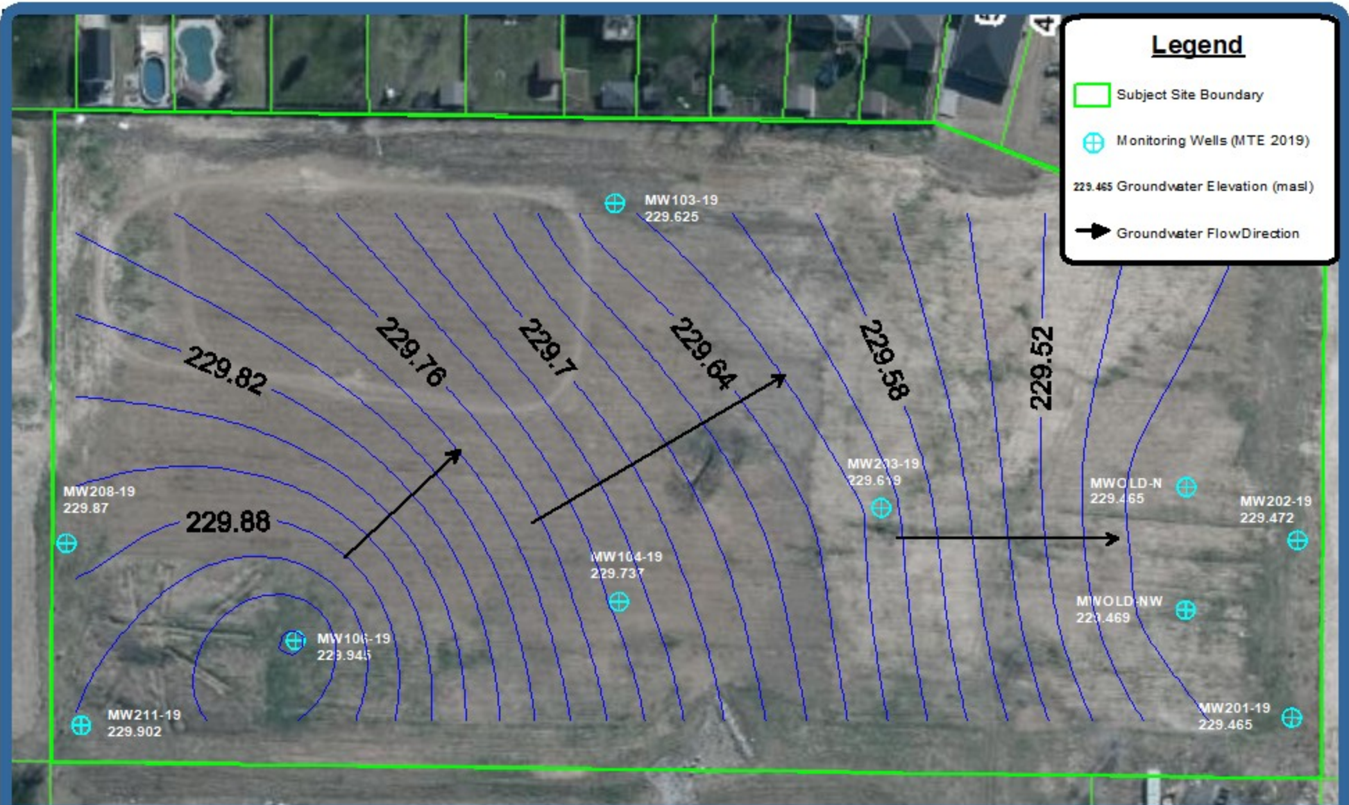
CSM Figure 6: Groundwater Contour and Flow Direction No Municipal Address, Darcy Drive, Strathroy, Ontario
