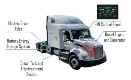
tered full-scale production following successful field trials. It combines a 270kW battery with a low-emissions diesel generator, offering quieter operation, regenerative braking, and emissions reductions exceeding 50%. The modular design supports route-specific power balancing and simplifies maintenance. New Way reports high interest from municipalities and private haulers seeking transitional decarbonization technologies.
