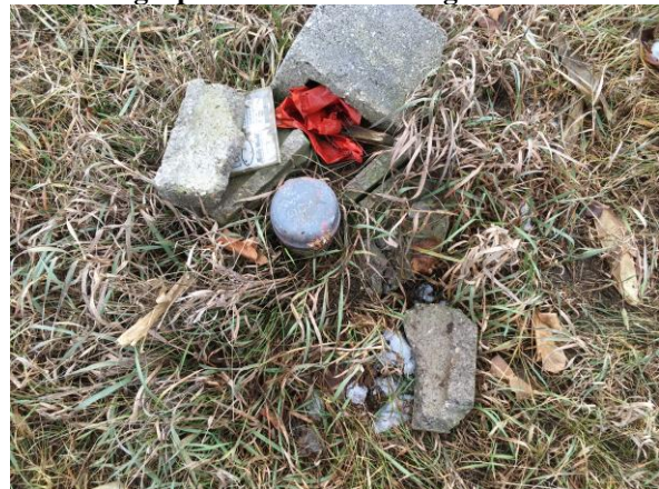
Photograph 4: Suspected filler pipe on northwest corner of the Site just south of the driveway
